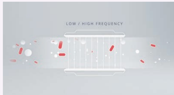
Microelectrodes in the microfluidic flow channel generate electrical fields at high and low frequencies.
